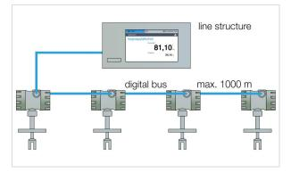
Controller with connection of maximum four sensors
