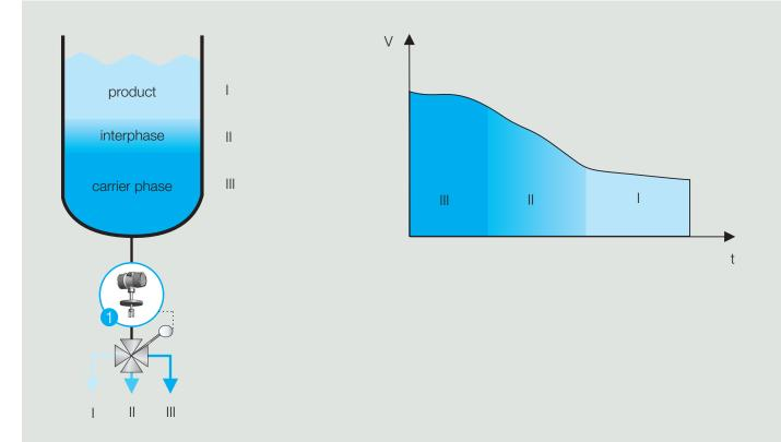
Phase separation in the batch process
