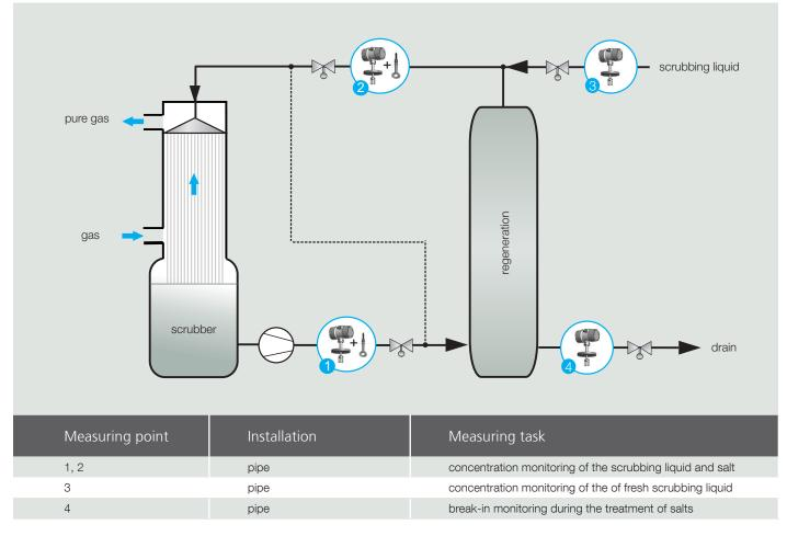
Gas absorption process in a jet scrubber
