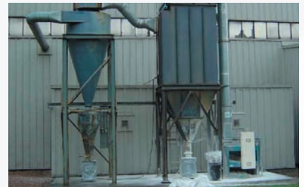
LEV (above) & Talc plant (below) monitored utilizing a networked Electrodynamic system
