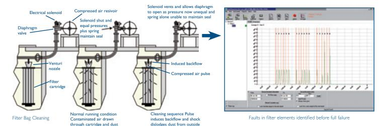
As a filter is reverse jet cleaned, any defects in the filter membranes are exposed resulting in relatively high dust peaks. By monitoring these peaks in real-time using PCME's Predict software package, it is possible to identify potential problems within the filter before they result in breaches of environmental limits. Marker pulses generated from the filter's cleaning system allows easy identification of damaged rows.
