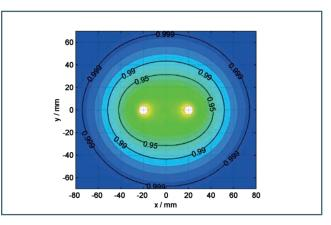
The figure shows the measurement field of the standard GR probe. The broad distribution of the measurement field up to 95% (green area) ensures optimal measurement results.
