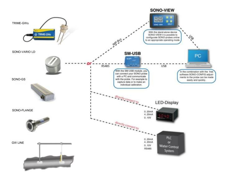
Predictive sensor networking through intelligent device communication ensures smooth processes in the application. The IMP bus does not transmit its data packets as voltage pulses, but as current pulses. Thus, the process works even with long cable lengths on existing and already laid lines. A shielded cable is not required and even spurs in wide-ranging network topologies are not a problem.
