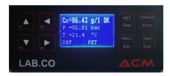
Sample loss-free and high precise CO, determination!
