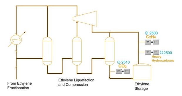
1) ② The ethylene product at the end of the process is monitored for residual  $CO_2$  traces to check purity. The ethylene purity is also measured (99.9%), and the level of any heavy hydrocarbons.
