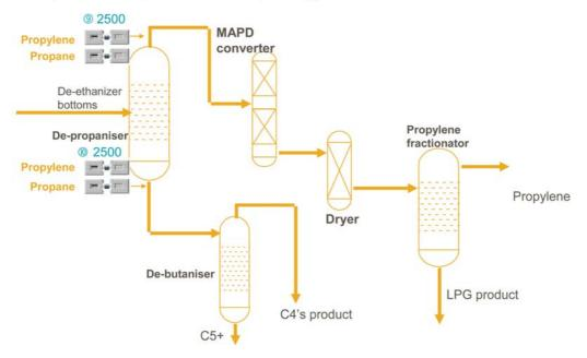
The de-propaniser separates C3's and C4's+. Then the propane is separated from the propylene in a fractionator. The de-propaniser bottoms are then sent to the de-butaniser to separate the C4's from C5's+
